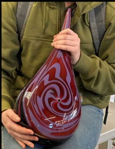
A sample of what our demo product would be like after 24hrs of annealing
